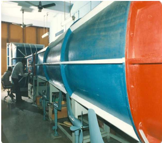
Wind Tunnel Range: 0 to 35 mps
