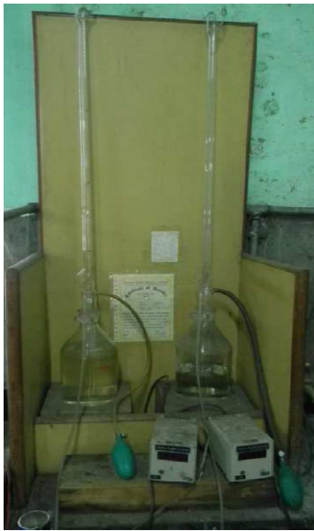
Standard Burette-pipette apparatus SRRG Calibration
