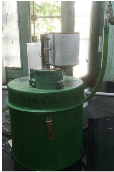
Standard Burette-pipette apparatus SRRG Calibration
